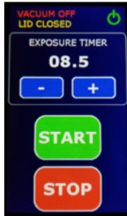
7. Enter the amount exposure time desired on the “Exposure Timer” by pressing the “ - ” or “ + ” buttons. Typical exposure times are shown below for a starting point. Brand of emulsion, screen mesh count, and thickness of emulsion applied will all effect exposure times, so some trial and error testing will be required. Start with exposure times in the middle of those shown below and adjust from there as required.
