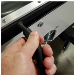
**WARNING:** When using an extension cord, use 14 ga. -3 conductor. Maximum length, 25' (7.62m).
