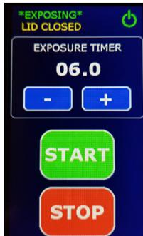
**NOTE: The START button, timer, vacuum and UV LED, WILL NOT FUNCTION until the lid is "Closed and latched" to ensure safety of the operator from the UV light source.**
