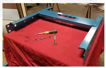
2. Remove the Spectrum unit from shipping box and place on two sawhorses as shown below. Sawhorses will need to be at least 30" tall.
