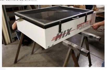
3. Install the two leg assemblies to the Spectrum using the 3/8" bolts and washers removed in the previous step. Note the "HIX" log should face outward as shown. Push the leg upward so that the tab on the leg is flush with the bottom of the Spectrum. Tighten all of the 3/8" bolts.
