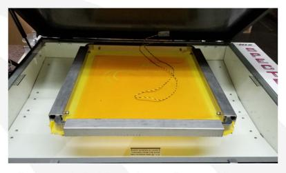
Drape the vacuum/anti static cord across the screen frame as shown.
