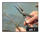
Using needle-nose pliers and flathead screwdriver works best when weaving the link splices together (pic 13b, c and d).
